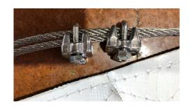
**Step 2** | Unwind tensioners all the way out and attach to the cover. Apply anti seize to thread of bottle screw.
